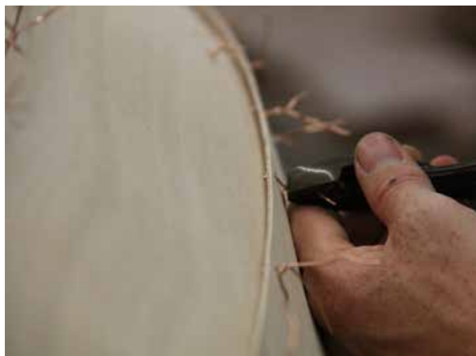
Here, the panel edge strikes a clean, fair curve from stem to stern.
