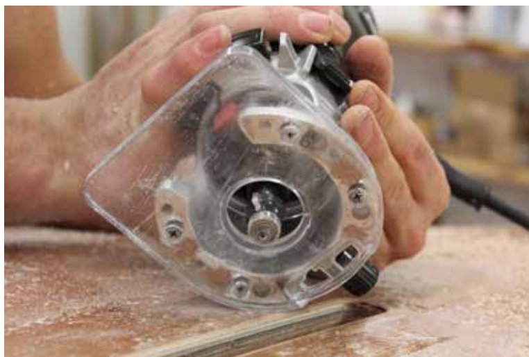
A bottom-bearing flush-trim bit.
