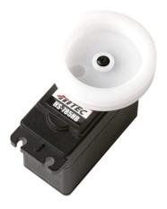
I recommend the Hitec Model HS-785HB sail servo which has a drum for winding the sail sheets mounted atop a self-contained motor-gearbox-control unit. The drum makes several rotations to adjust the sails from full-in to full-out. The Instructions from CLC describe the installation of this winch.
