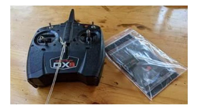
To set up the radio for sailing, you will have to do some modifications. The transmitter control sticks should be modified to allow you to control the in and out of the sails.
