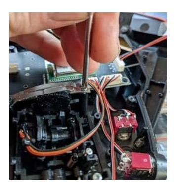
This is easily done by removing the back of the radio transmitter and turning a screw on the left hand up and down stick to relax the spring which centers the stick and to tighten the ratchet spring which holds the stick where you set it. See page 11 of the manual (for English.)
