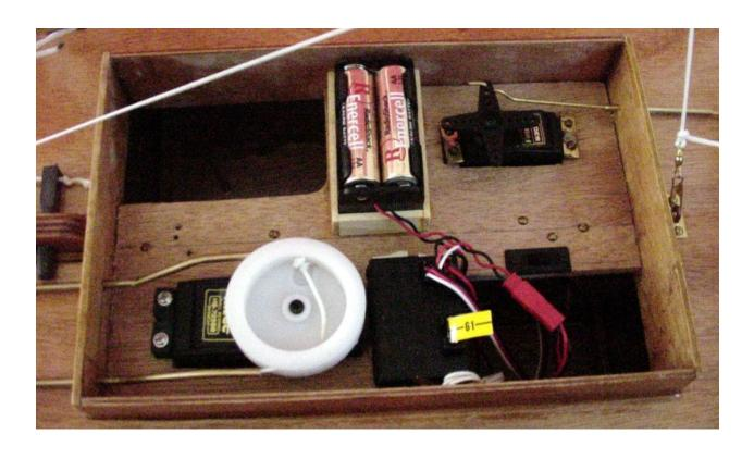
I plug the battery into the battery slot on the receiver, the sail winch into slot #1 and the steering servo into slot #2.
