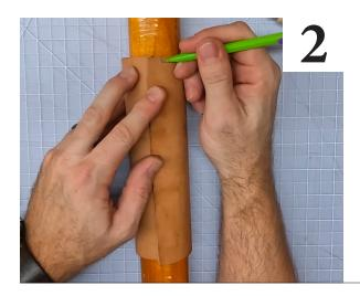
**Trimming the Collars:** Using the center location in step one, align the center of one edge of the leather so it runs lengthwise on the oar shaft. Wrap the leather tightly around the oar, hold it in place and mark both ends 1/8" inside of the leather overlap. Lay the leather flat, mark the cut line, and cut off the excess material with a razor knife.
