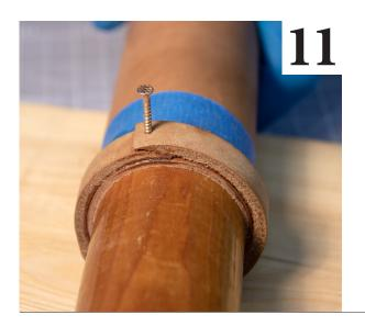
**Nail Down the Button:** To secure the button end, install a single ring nail at the end of the button. Carefully tap the included ring nail in place. Only use one nail for each button.
