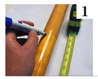
**Find the Center of the Collar:** Distance to the center of collar = Distance between oarlocks, divided by 2, plus 2 inches.
