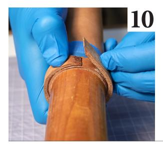
**Installing the Buttons Continued:** Carefully wrap the button around the collar, pressing in place. Contact cement is strong glue and will instantly hold it in place.
