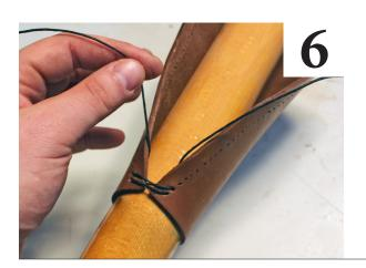
**Gluing & Stitching:** Apply contact cement to the inside of the collar. Using the location from step 1, wrap the collar around the oar shaft aligning the stitch line lengthwise with the oar shaft.
