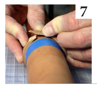
**Scarf the Buttons:** The button is the thin strip of leather located at the top of the handle end that helps keep the oar lock in position. Cut a scarf at one end of the button with a razor knife or sharp chisel (as seen in the picture). Wrap the button around the top of collar, then mark and cut a scarf at the opposite end. This will help with the button fit. Repeat with the 2nd button.
