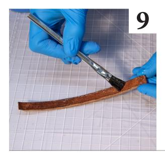
**Installing the Buttons Continued:** Apply contact cement to the mating surfaces of the oar collar and the button. Allow the contact adhesive to dry, per glue instructions.
