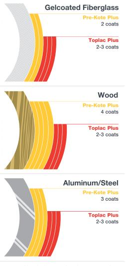
For a good level of protection, Interprotect is no longer required on metal substrates. However, if additional levels of protection are required then one coat of Interprotect, thinned with 10-15% of 2316N Reducing Solvent can be applied, followed by two coats of Pre-Kote Plus.
