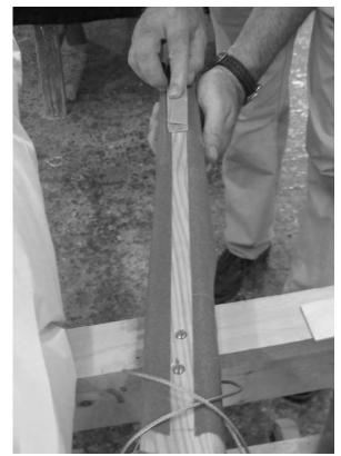
Epoxy should be thickened to a mustard-consistency paste and applied to the batten.
