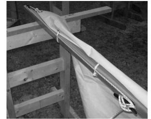
You will need to install a new cleat for the main halyard on the side of the mast. We put ours a few inches down from the gooseneck. Use #8 x 1-1/2" (38mm) silicon bronze screws.
