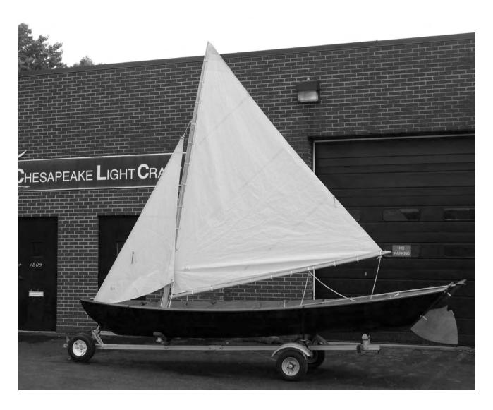
The sloop-rigged Northeaster Dory. Could use a little more downhaul tension, or a little less outhaul tension, to take that wrinkle out of the foot of the sail.
