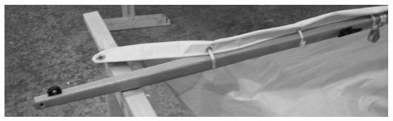
The foot of the mainsail is still laced to the boom per the stock version---don't be tempted to use this particular sail loose-footed. However, the lacing should be loose enough to allow the foot of the sail to slide on the boom.
