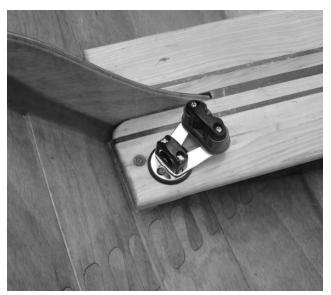
Here's a view of both swiveling cam cleats in place
