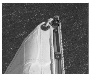
The mast track is screwed to the mast with #6 x 3/4" (18mm) screws.
