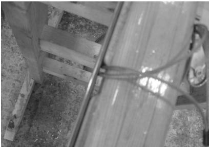
An outhaul for the mainsail is added to improve sail shaping, to make it easier to drop the boom when the halyard is loosed, and to facilitate reefing if that option is chosen.
