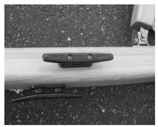
You will need these slides fastened in the grommets along the luff of the mainsail so that it can slide on the track.
