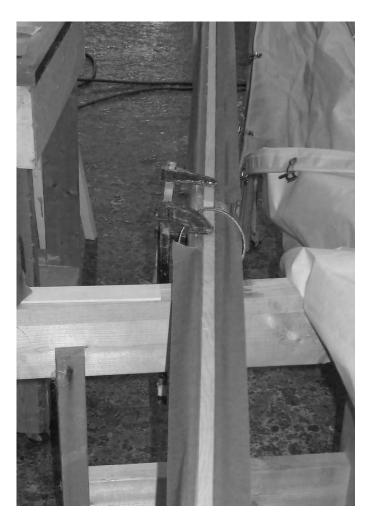
Here's the rest of the batten clamped to the mast, epoxy curing.
