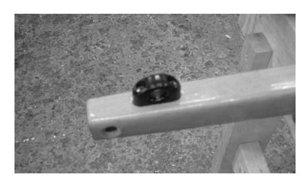
Further forward on the boom, within easy reach, you'll install a 4-inch (100mm) cleat with two #8 x 1-1/2 (38mm) silicon bronze screws.
