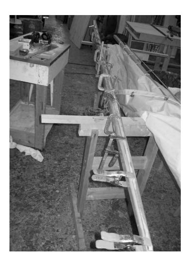
Once the epoxy has cured, remove the clamps, sand the batten smooth, and apply layers of epoxy and varnish. Notice we've protected our varnished mast with more masking tape.
