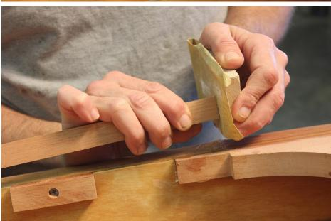
Find a helper for this step, then spread thickened epoxy on the spacer blocks.
