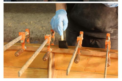
With both inwales in place, sand the tops of the rails flush. Make sure you don't over-sand and turn the boat's sheer into a wavy line.
