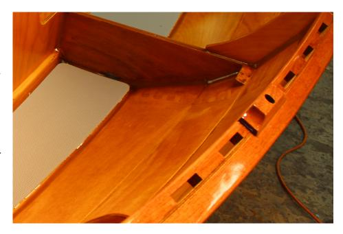
little wooden blocks elevating the rail off the plywood. Spacered inwales are a new invention, mostly unknown until maybe 30 years ago. What the spacer blocks are doing is imitating the tops of the steam-bent frames in traditionally-built boats. Functionally, the spaces create solid tie-off points around the perimeter of the boat, very handy indeed.
