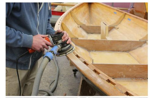
A router with a round-over bit is one way to ease the edges of the inwales and outwales. If the router bit is dull, or if you try to cut too much in one pass, there's real danger of picking up a "running splinter" that breaks a rail in two. Proceed with caution, and use a sander to create the round-over.
