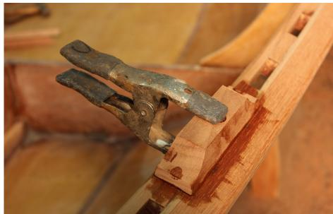
So that the top mount oarlock sockets will seat properly, you'll need to drill out the inwale assembly to match the hole in the oarlock riser.
