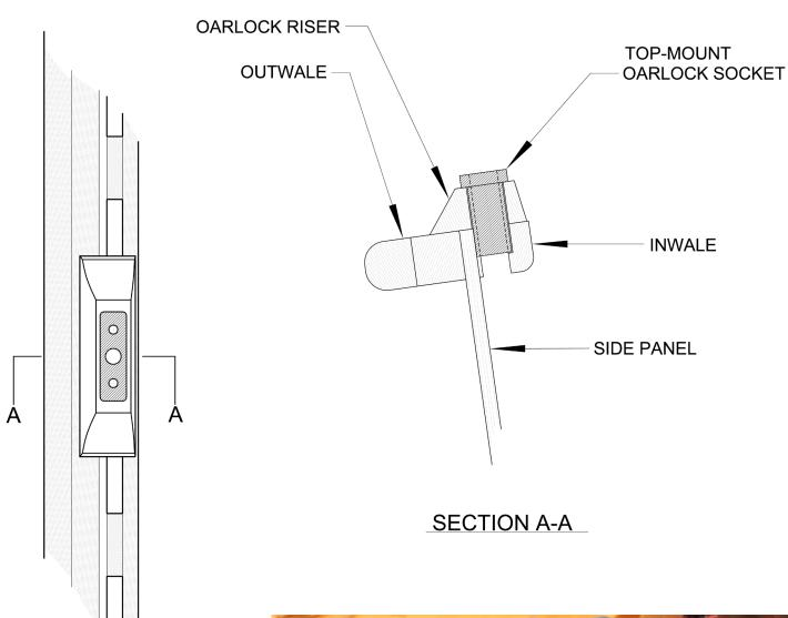
The addition of spacered inwales complicates the installation of oarlock sockets. Quite a lot!
