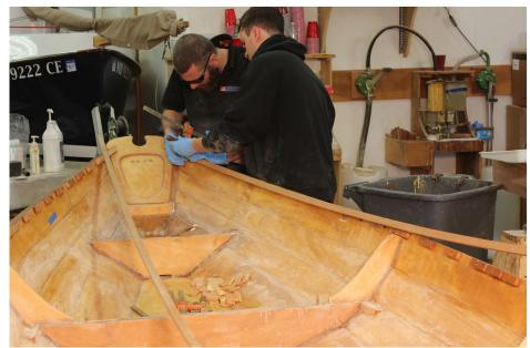
...and work your way forward, making sure the inwale is flush with the top of the hull.
