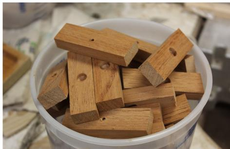
The spacer blocks may be clamped in place while the epoxy cures. However, we elected to use screws to install the spacer blocks.
