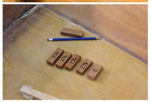
Spacer blocks are located and marked along the length of the hull.
