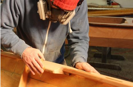
Knowing the abuse our demo model Northeaster Dory will endure, we elected to add an epoxy fillet for extra strength where the mount rests against the hull.
