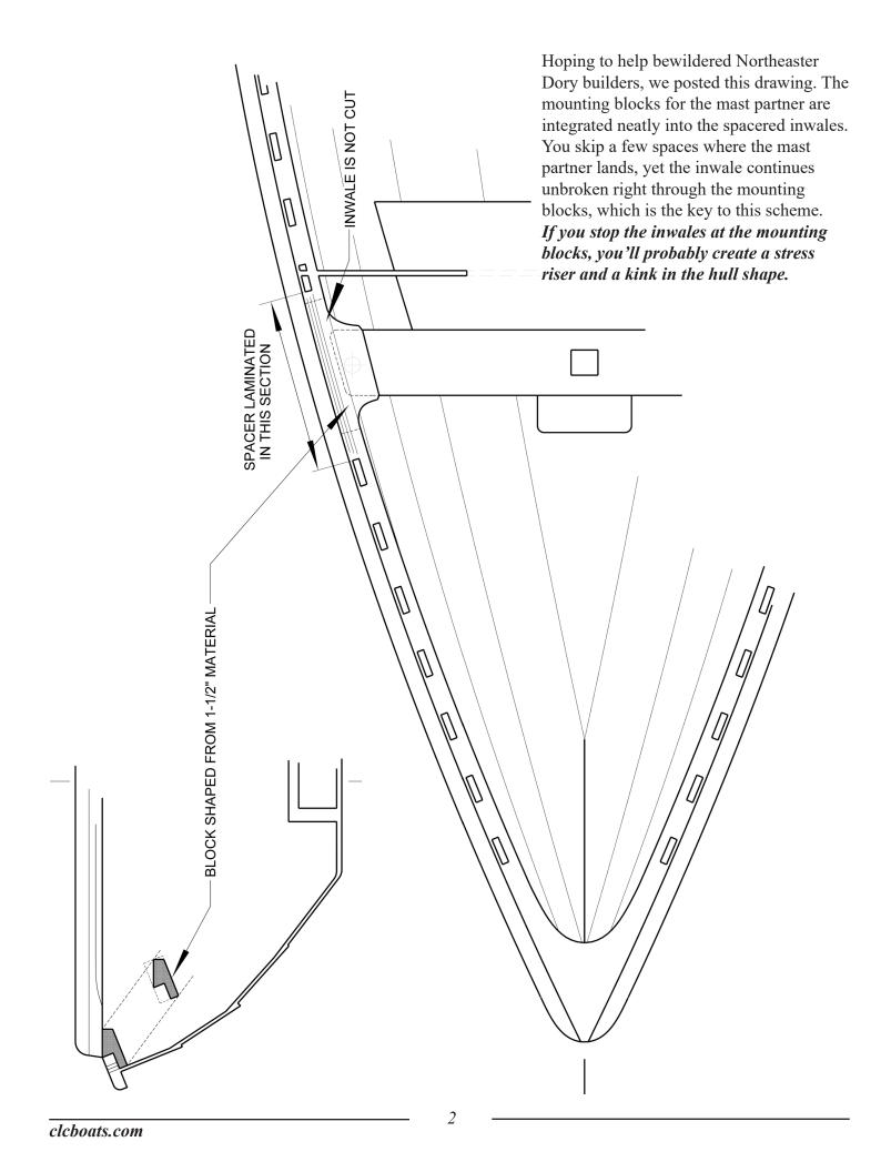
We retrofitted Northeaster Dory Hull #1 with spacered inwales, in part because it was old and in need of cosseting, but also to capture photography of how this odd business of lug rigs and spacered inwales fit together.
