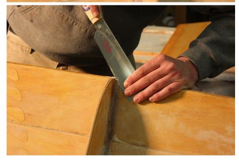
The notches in the three frames have been opened and checked.
