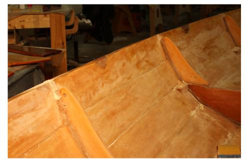
Time to figure out the spacing for your spacered inwales!
