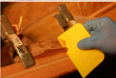
Sand the tops smooth. A straightedge spanning the hull should rest flat atop the mounts.
