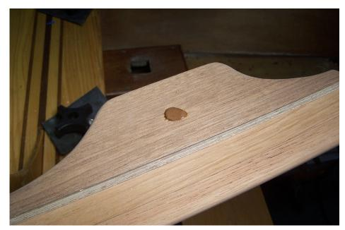
....then drill again with a 3/8" (9mm) bit for the bolt. The epoxy protects and strengthens the holes in the T.L.R.N.D.S.I. mounts.
