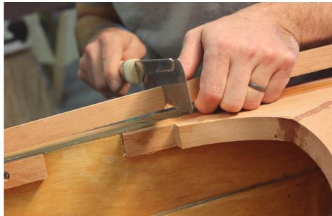
We made it just a hair too long, and a couple of swipes with a sanding block resulted in a tight fit.
