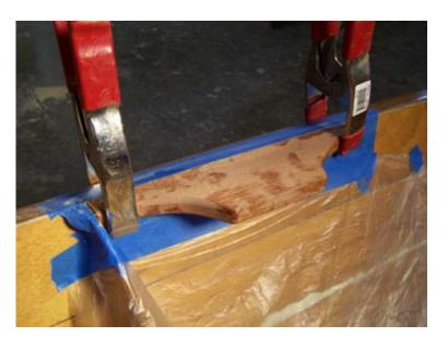
Note the trouble we took with plastic and tape, to avoid dripping epoxy on the varnished interior of our showroom model.
