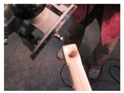
The boom and yard need 5/16" (8mm) holes at each end, centered about 1" (25mm) from the end of each spar.
