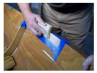
Thicken epoxy with Cell-o-fill and brush a heavy coat onto the knees.
