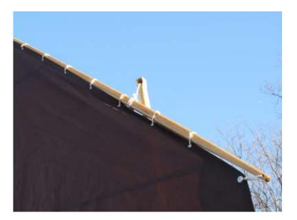
Here's the downhaul, which not only helps tension the sail in the vertical dimension, but also holds the boom in the correct orientation. Again, the exact amount of tension is an artform, but should default to being very tight.
