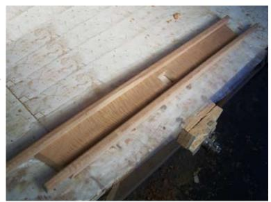
Thickened epoxy is applied to the mating surfaces....
