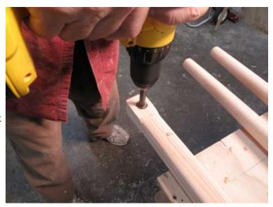
The halyard needs to run smoothly though the hole. We used a router and a round-over bit to "flare" the hole neatly. Thus treated, there is almost no friction on the halyard.
