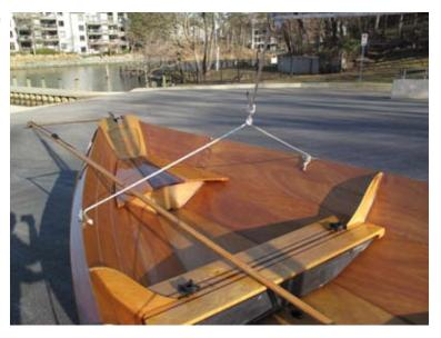
In the middle of the bridle, create a loop and an overhand knot.
