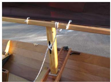
The main sheet is rigged to a bridle. The oarlocks at the rear rowing station are perfectly placed for the bridle; we just passed a length of 1/4" (6mm) line into each oarlock and tied a knot.
