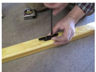
The cleats are positioned on the port and starboard faces of the mast.
