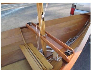
A view of the halyard in action. You should hoist the sail first with the halyard, then take up on the downhaul.
