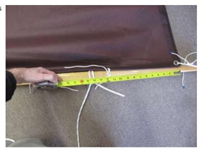
Halyard and downhaul are 1/4" (6mm) low-stretch line. Here's the knot we used, a clove-hitch around the spar followed by two half-hitches.
