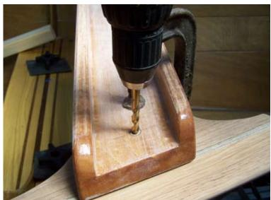
We will use the "drill-fill-drill" scheme to make sure these holes are strong and the bolts don't wear on the wood.
