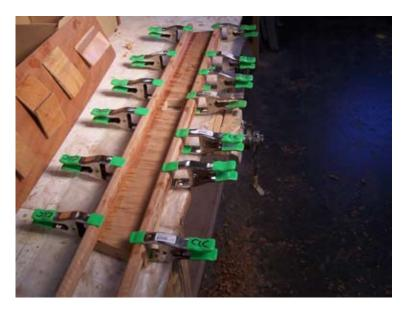
Double-check and triple-check against the boat that your thwart is the right length and that the angles are correct, then trim the thwart assembly to length.
