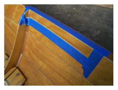
Every trace of varnish must be sanded away if you're retrofitting. If you're working on a hull that just has an epoxy coating, you still must scuff up the mating surfaces for the strongest-possible bond.
