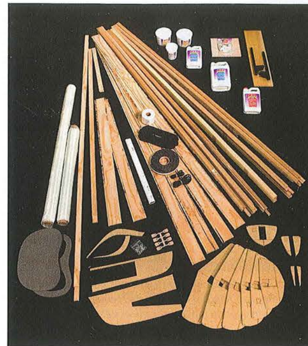
Left—Along with the major wood structural members and planking, each kit contains the epoxy and filler, fiberglass reinforcements, and specific fittings or hardware required for construction. The kit's completeness and logistical organization, allowing each one to be packed efficiently and consistently, deliver Ikea-like simplicity of construction. Above—The CLC mill shop turns out bead-and-cove wood strips for planking in numerous kits.
