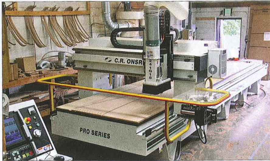
The new $230,000 C.R. Onsrud CNC machine installed in summer 2014 is more efficient than the one it replaced, and can affix bar codes to each component to aid in managing inventory. It will also be employed to cut kits for other designers.
