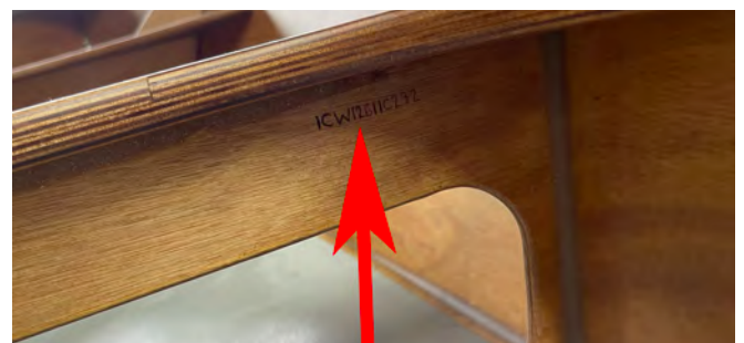
The Duplicate HIN on this Peeler Skiff is on a bulkhead beneath a seat.
