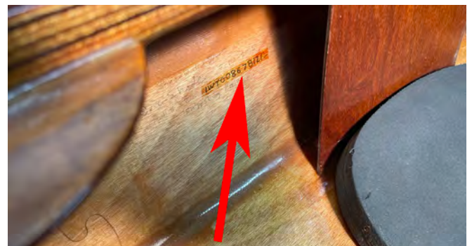
On kayaks, the Duplicate HIN is generally located in the cockpit. This one was written in pencil and over-coated with epoxy.
