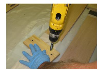
Don't have a wooden surface for screwing down clamping pads? Working on a panel wider than a few inches? You can use heavy weights, like buckets of sand, cinderblocks, or some free weights, spread across a board over the joint to distribute the weight evenly. It always takes more weight that you think. Just be sure to protect the floor or bench and whatever you use to clamp the joint with plastic.
