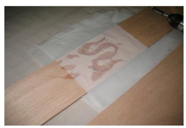
Blocks of scrap wood, protected from the epoxy with plastic and screwed down to a table top over each puzzle joint, provide the best chance of clean alignment and strong joints. on narrow panels where the scrap wood can span the joint without bowing to maintain an even pressure across the joint.
