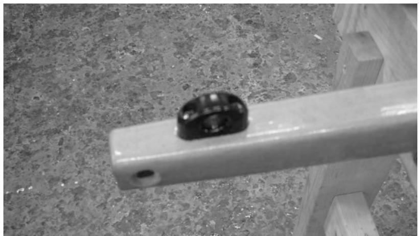
Further forward on the boom, within easy reach, you'll install a 4-inch (100mm) cleat with two #8 x 1-1/2 (38mm) silicon bronze screws.
