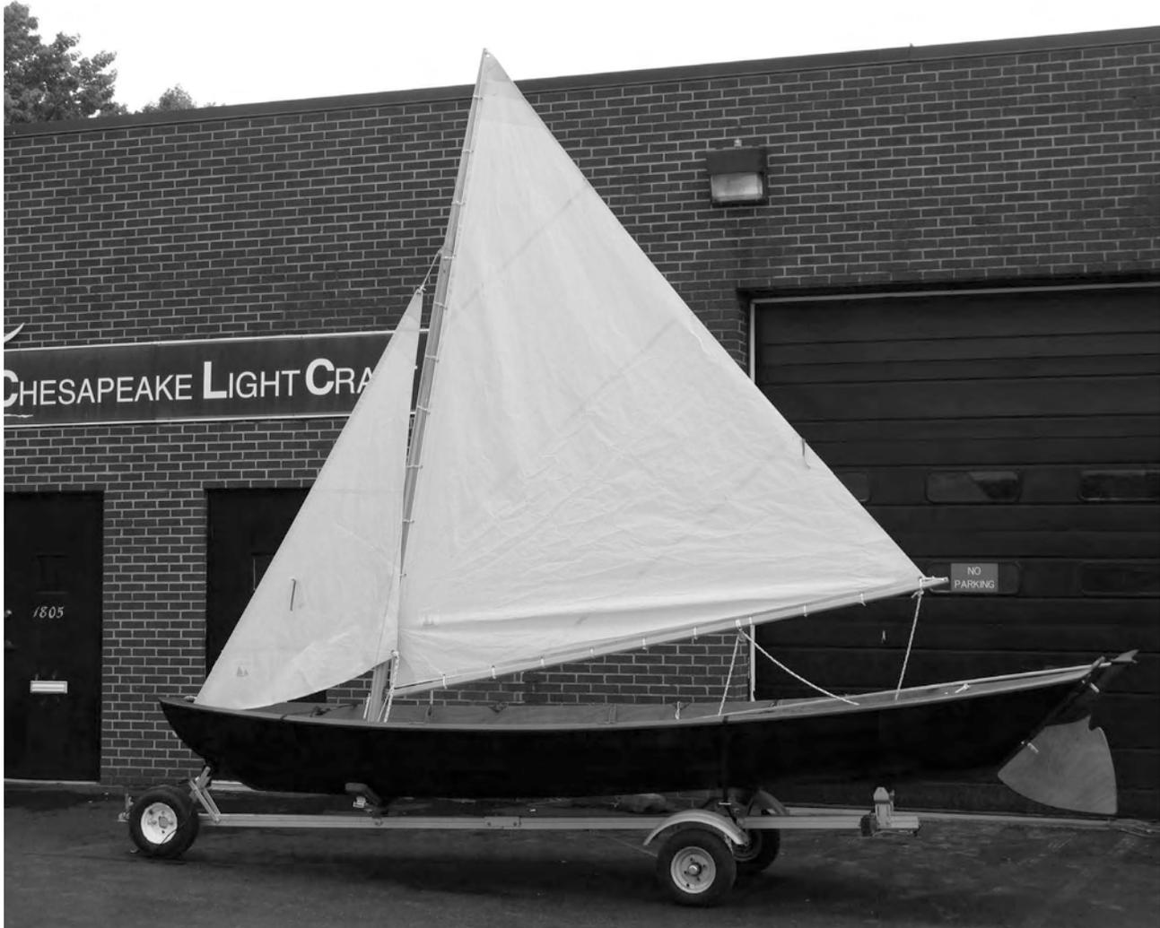
The sloop-rigged Northeast Dory. Could use a little more downhaul tension, or a little less outhaul tension, to take that wrinkle out of the foot of the sail.
