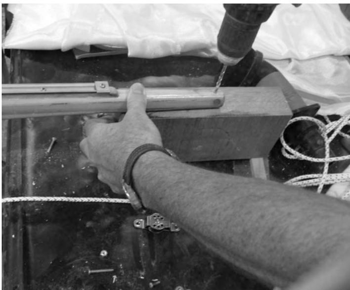
As always, put a dab of caulk in the screw holes before fastening the cheek block permanently.
