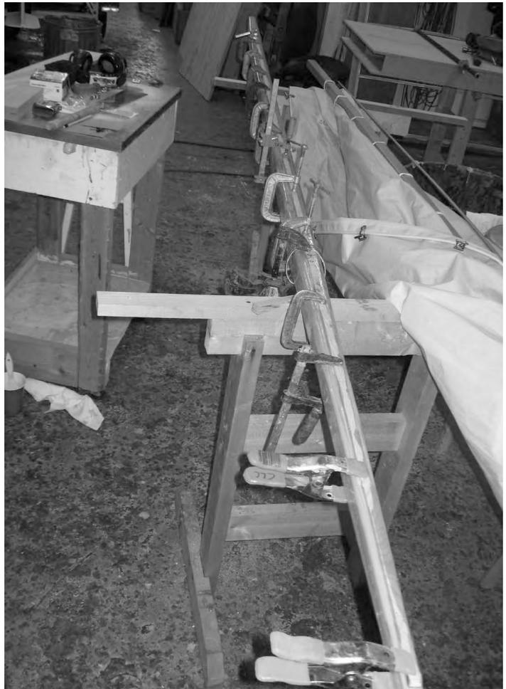
Once the epoxy has cured, remove the clamps, sand the batten smooth, and apply layers of epoxy and varnish. Notice we've protected our varnished mast with more masking tape.
