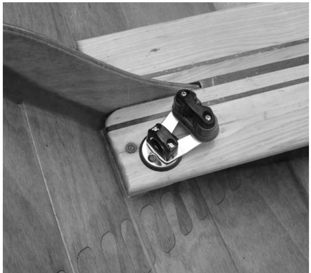
Here's a view of both swiveling cam cleats in place
